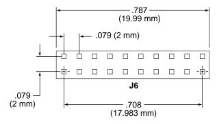
Figure 15. J6 connector dimensions
