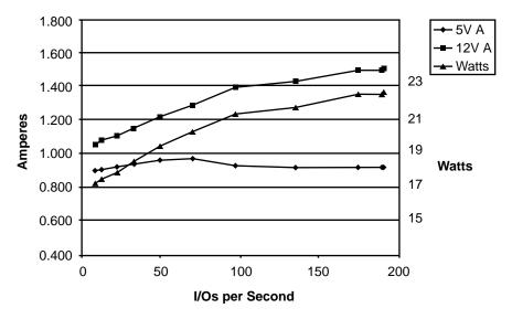
Figure 5. DC current and power vs. input/output operations per second
