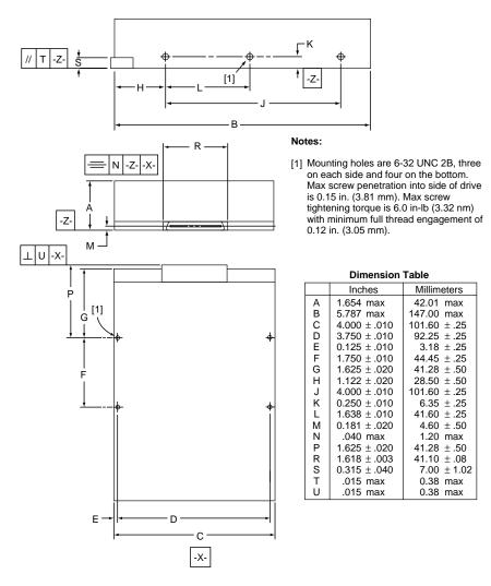
Figure 8. Mounting configuration dimensions
