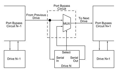
Figure 13. Port bypass circuit physical interconnect
