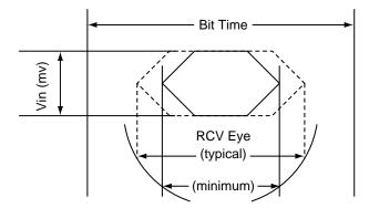
Figure 18. Receive eye diagram
