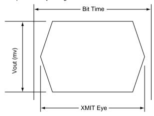
Figure 17. Transmit eye diagram
