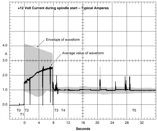
Figure 3. Typical Cheetah 73FC drive +12V current profile
