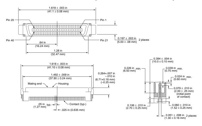
Figure 14. FC-AL SCA device connector dimensions
