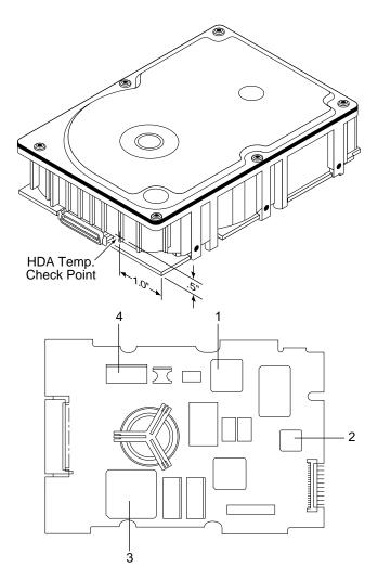
Figure 6. Locations of PCBA components listed in Table 2
