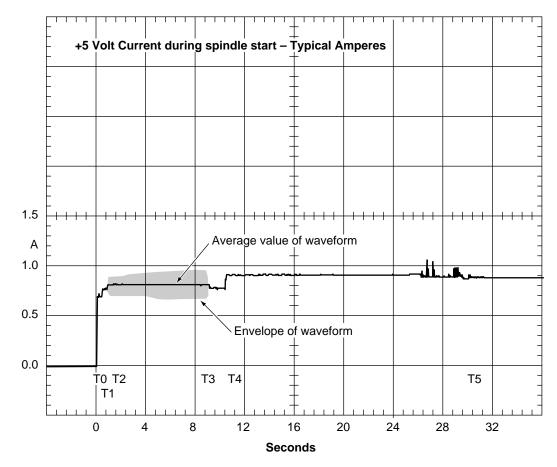
Figure 4. Typical Cheetah 73FC drive +5V current profile
